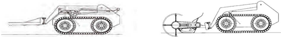
a) The vehicle with sensory platform b) The vehicle with flailing activation mechanism
