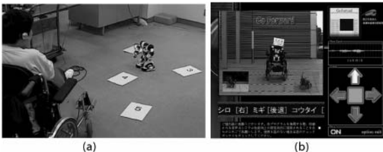
Fig. 5. Speech recording environment (a) Voice operated toy robot system (b) Graphical simulation demo system
