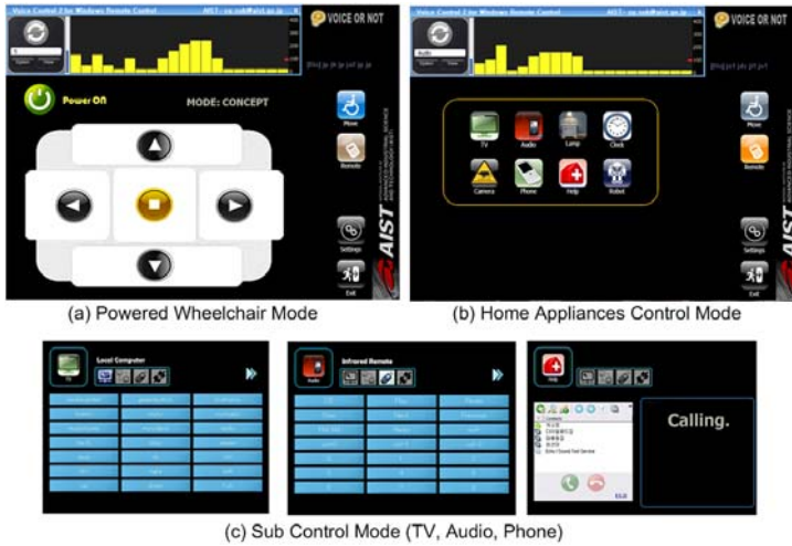
Fig. 7. Example of system GUI design (a) Powered wheel chair mode (b) Home appliances control mode (c) Appliance control sub mode
