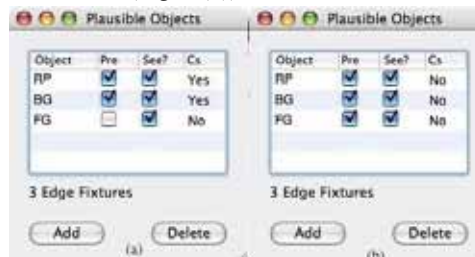
Fig. 6. Whether an Object is visible is indicated by See? for the current frame and by Pre for the previous frame. Column Cs shows whether the corresponding object is concluded to be consistent. (a) The two persistent landmarks ( RP and BG ) are consistent with each other, but inconsistent with the front goal ( FG ). (b) Nothing is consistent in this view
